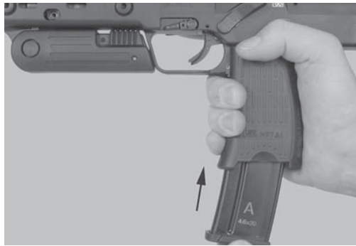
Fig. 15: Insertion of the magazine
