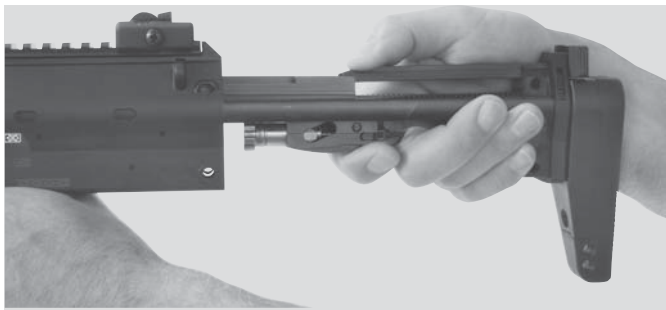
Fig. 36: Assembly of receiver, backplate with butt stock and bolt
