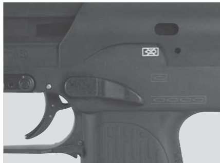
Fig. 13: Safety/selector lever at "BURST-FIRE"
