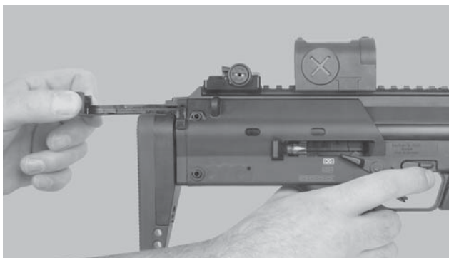
Fig. 17: Arresting the bolt in the open position
