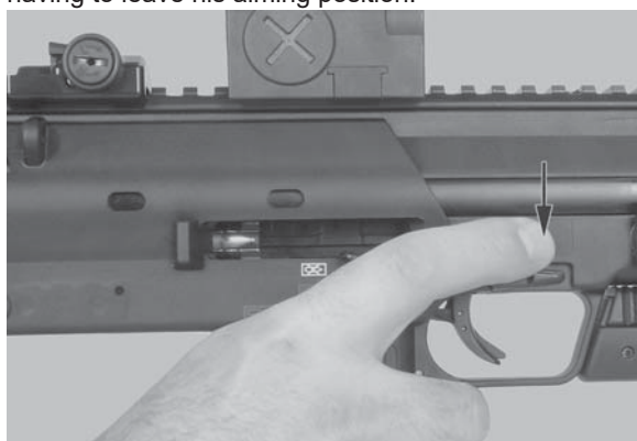
Fig. 17: Release of the bolt by actuating the bolt catch/release lever
