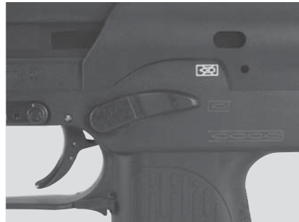
Fig. 12: Safety/selector lever at "SEMI-AUTO"
