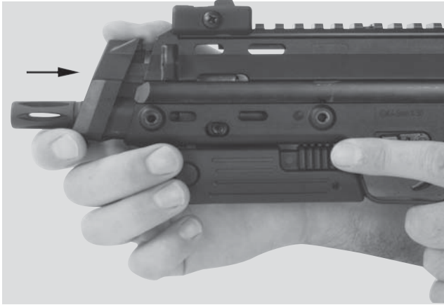
Fig. 37: Slide the front cover onto the receiver
