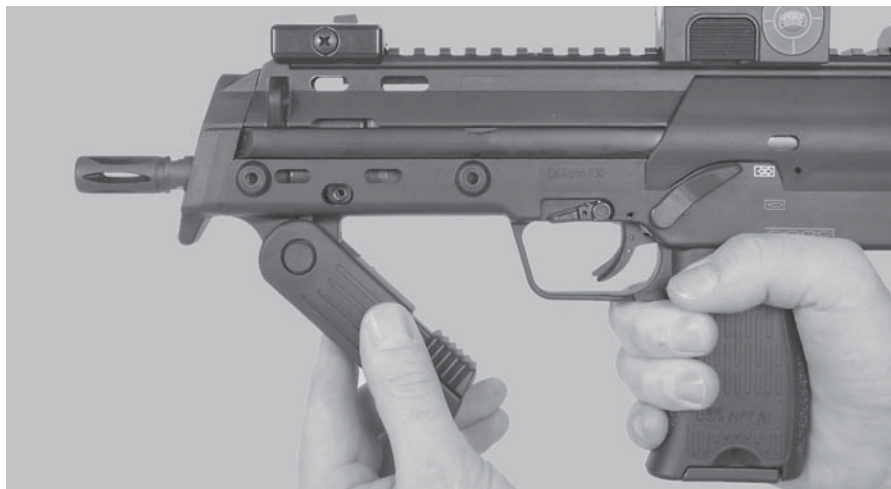
Fig. 9: Extending of the locking grip
