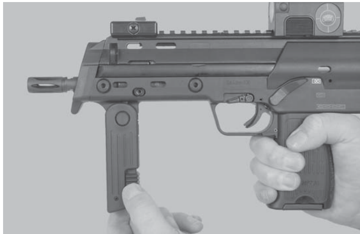
Fig. 10: Unlocking of the folding grip release mechanism
