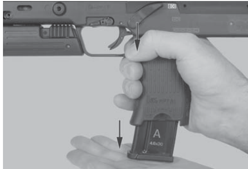
Fig. 14: Actuation of the magazine catch for removing the magazine
