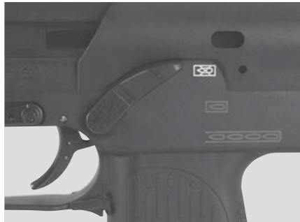
Fig. 11: Safety/selector lever at "SAFE"
