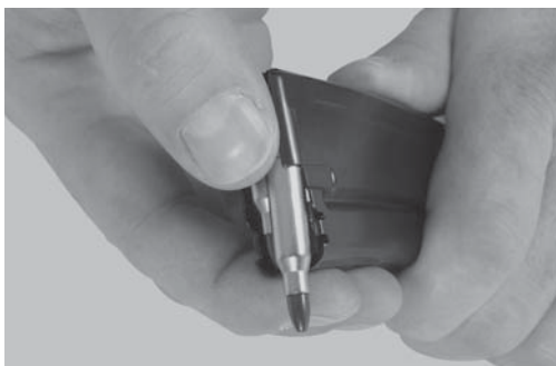
Fig. 20: Unloading the magazine
