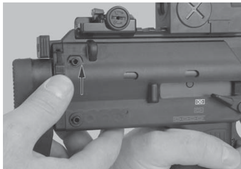
Fig. 7: Unlocking of the retractable butt stock
